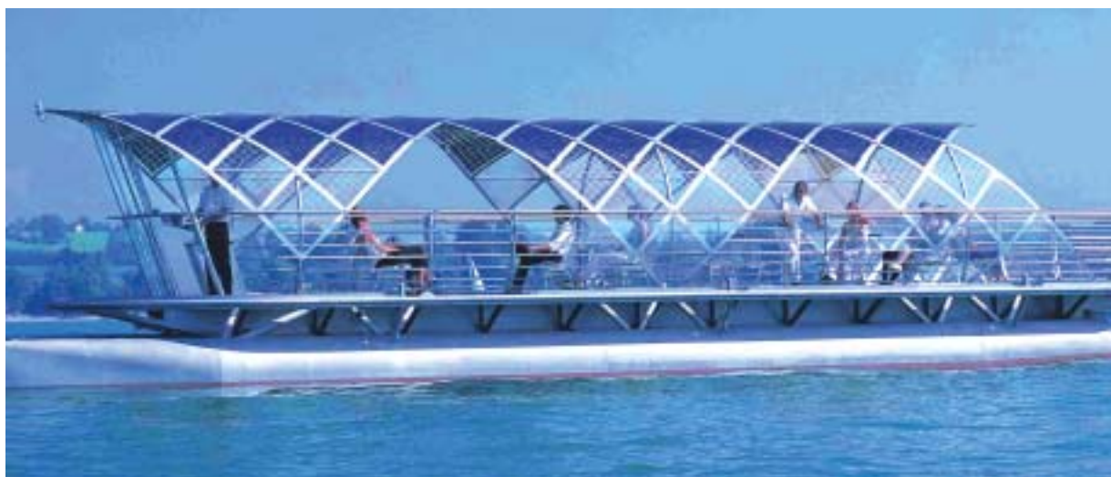
Emission-free solar power boats such as the solar ferry „Helio“ at Lake Constance are operating at the Broads and several other lakes and rivers in the world.
